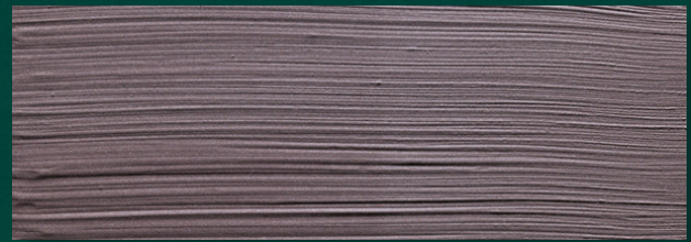
A traditional primer with an uneven film thickness due to its poor flow characteristics
